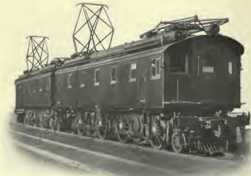
FIG. 540. ELECTRIC LOCOMOTIVES. Locomotive for 11,000-Volt Single-Phase Overhead Contact Operation, Norfolk & Western Railway.
